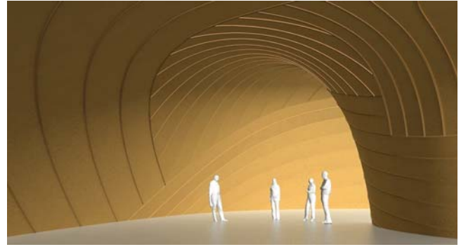
Figure 5: Geodesic D-strip models (in total five) which cover the interior of a freeform surface.
