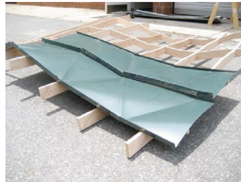
Figure 4- Standing seam test on frame
