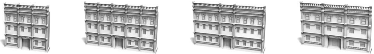
Figure 7: Structure discovery and procedural modeling on a building facade. The regularity patterns of the model on the left have been extracted automatically and can be modified by the user to alter the facade design as shown in the middle. For comparison, the image on the right shows the original model scaled along the horizontal axis.
